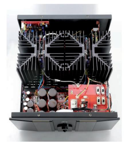
heat. As for output, the BSC-100m can produce a power of 100W when the matching speaker's impedance is maintained at  $8\Omega$ . If a pair of  $4\Omega$  speakers is used, such as the Dynaudio Confidence C4 signature version at our audition room, output figures will be instantly doubled to 200W. Even if it drops to  $2\Omega$ , or  $1\Omega$  which is near short circuit, the manufacturer guarantees that the output figures will not be lower than 400W and 800W respectively.
